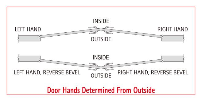
The door handing (left or right) is determined from exterior or outside of door (secure/key side). Exterior and interior handles are defined as follows:
